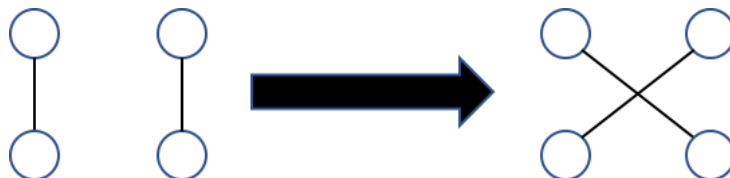
Figure 6 Edge-swapping to produce random versions of a network with the same degree distribution
