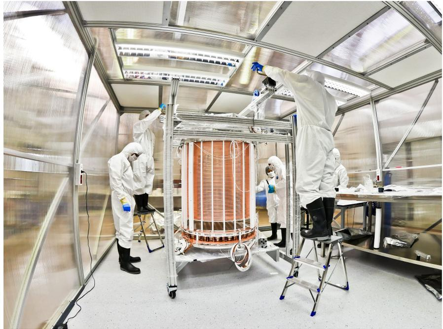
**Figure 15:** The heart of the XENON1T apparatus being assembled in the clean room. (Image credit: XENON1T.)
